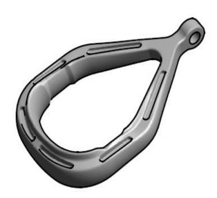
The Permanent Chain Chaser is used on semi-submerged rigs to prevent anchors from having to be buoyed off for recovery. The material of the Permanent Chaser is softer than the wire or chain. This is to make the chaser sacrificial between the two so that the chain or wire does not get damaged. This is used as an alternative to the buoy and pennant.
